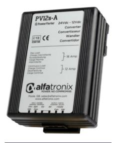
Alfatronix have developed three voltage converters, a 3Amp, 6Amp (continuous) and a 12A (continuous), which overcome these configuration problems. The Alfatronix converters mimic the 12V battery and 12V ignition function by providing two outputs, either of which can provide full power. One output is available whenever the 24V battery is connected. The other output is switched by the 24V ignition switch. Now the ICE equipment can be fitted to the 24V truck as simply as fitting it to a 12V car.
