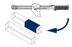
■ It is not necessary to keep the tool set at the minimum load after use
