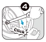
Hold the handle firmly in the middle and use the torque wrench clockwise. Stop immediately after "click".
