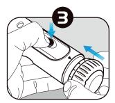
Press the safety button and simultaneously press the adjustment ring.
