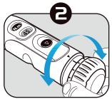
Turn the adjustment ring to adjust the desired value on the scale with convex lens.
