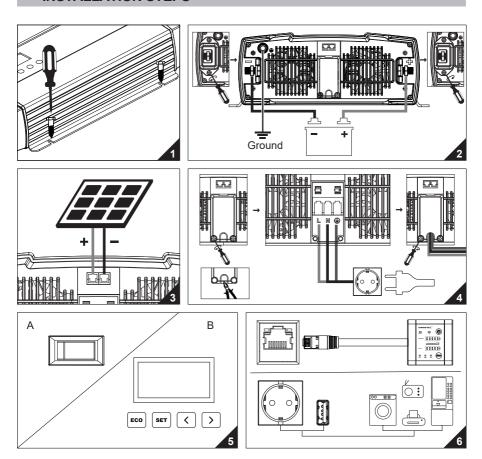
Step.1: Position screws into mounting holes to fix the inverter properly.
