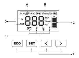
A.ECO/Solar/UPS Functions B.Setting Options C.Battery Electricity Status D.Parameters Display E.Fault Icons F.4 Buttons Control
