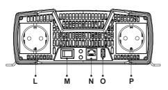
L: AC Socket 1 O: USB Port M: ON/OFF Switch P: AC Socket 2
