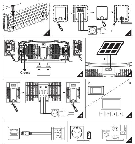
Step.1: Position screws into mounting holes to fix the inverter properly.
