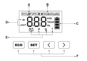
A.ECO/Solar/UPS Functions B.Setting Options C.Battery Electricity Status D.Parameters Display E.Fault Icons
