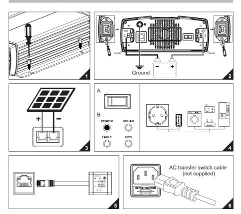
**Step.1:** Position screws into mounting holes to fix the inverter properly.
