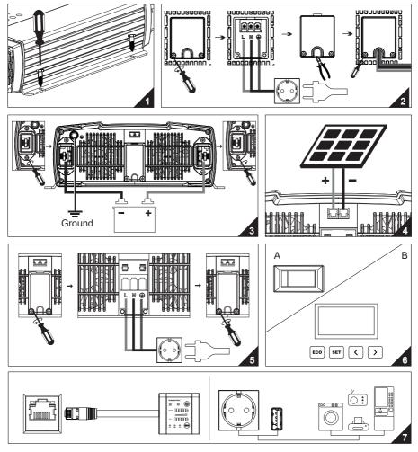
Step.1: Position screws into mounting holes to fix the inverter properly.
